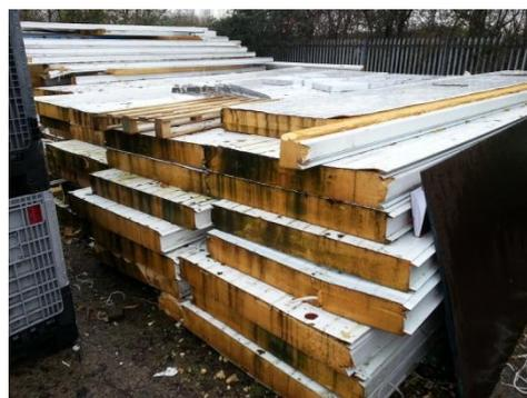
The dismantled cold store was made up of 80 panels measuring 8 metres long, 120cm wide and 10cm thick. Infrastructure for recycling insulation is very limited and any recycling programme would have meant transporting two articulated lorry loads of panels across the country. Using insulation to generate energy is not efficient as insulation is typically treated with fireproofing chemicals.
